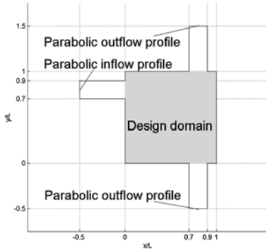
(a) Boundary conditions (D). The velocity profile is prescribed at the boundary and the design domain is colored grey. At edges without a label the no-slip boundary condition is enforced.
