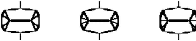
Figure 3. Topologies obtained considering constant, linear, and quadratic output springs.
