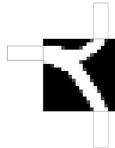
(d) Using the BCs in Figure 1(c), the rate of energy dissipation is minimized with a constraint on the difference between the outflow rates.
