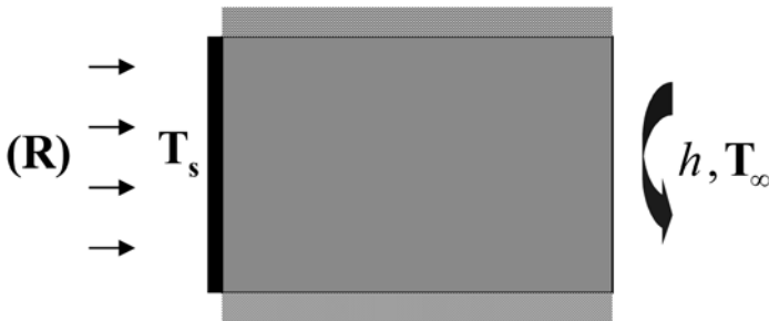
Figure 6. A simple heat transfer system illustrating energy balance.
