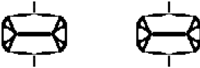
Figure 2. Topologies obtained for the linear (left) and nonlinear (right) cases, using filtering.
