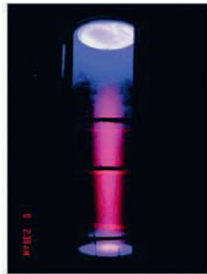
Figure 5. Photograph of the large glow discharge tube at a pressure of 1.2 Torr (160 Pa) and a current density of 6.6 A/m 2 . At this pressure, the positive column is restricted relative to the tube diameter.
