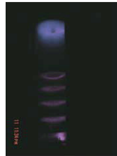
Figure 6. Snapshot photograph of the large glow discharge tube at a pressure of 70 mT (9.2 Pa) and a current density of 0.12 A/m 2 illustrating quasi-periodic striations, uniformly distributed across the tube at this pressure.
