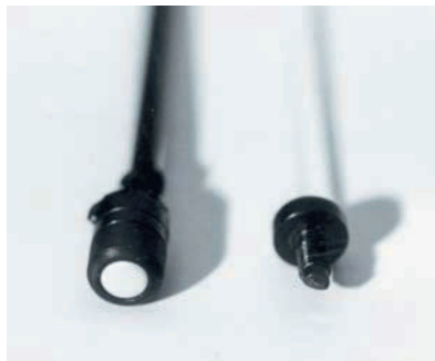
Figure 7. Photo of the CO 2 -probe head used in the clinical validation.
