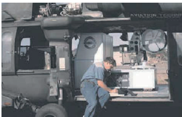
Figure 1. US Army's Long Range Standoff Biological Detection System operates off a Black Hawk Helicopter and uses LIDAR to detect changes in particle concentration 2 .
