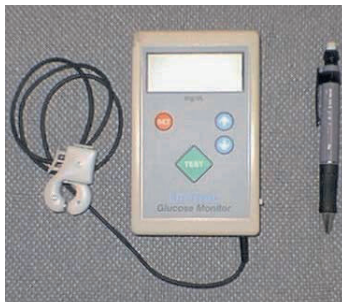
Figure 11. Photo of the prototype of the glucose sensor developed by Lifetrac.
