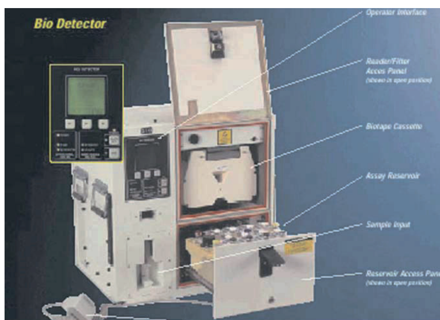
Figure 4. The Bio-Detector performs 8 immunoassays simultaneously and is currently marketed by Smiths Detection (Edgewood, MD).
