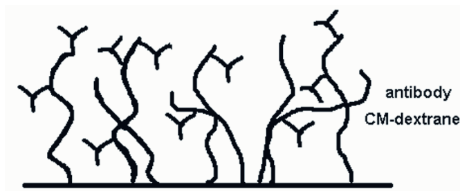
Figure 5. The binding of antibodies to carboxymethyl dextran matrix attached to a sensor surface.
