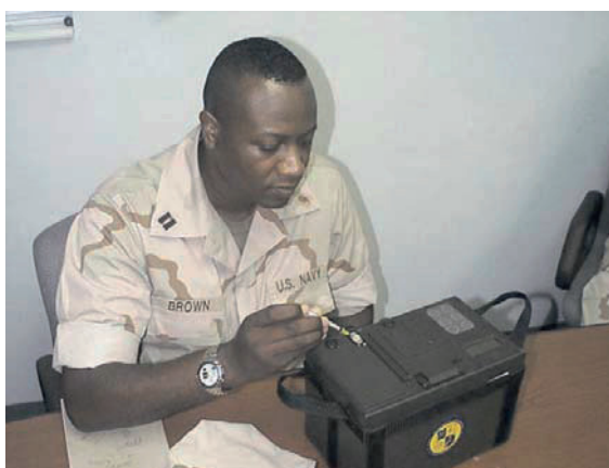
Figure 6. US Marine using the RAPTOR to test for toxins and pathogens in drinking water in Bahrain.
