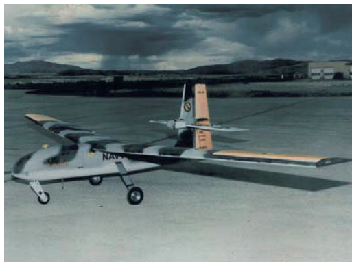
Figure 5. The unmanned plane used to collect and identify aerosolized bacteria in field trials at Dugway Proving Ground, UT. The plane carried a ten-pound payload including a cyclone air sampler and 4-probe fiber optic biosensor.
