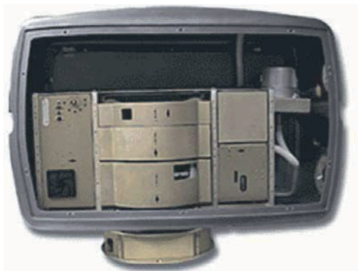
Figure 3. Recent version of the Portal Shield system housed in a temperature controlled chamber for long-term monitoring around fixed sites ( www.dcfp.navy.mil/cbrd/ca/actd.htm , March 20, 2004).
