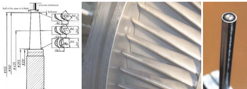
Figure 6. Rotor geometry (a) and the position (b) of the unsteady pressure transducer (c)
