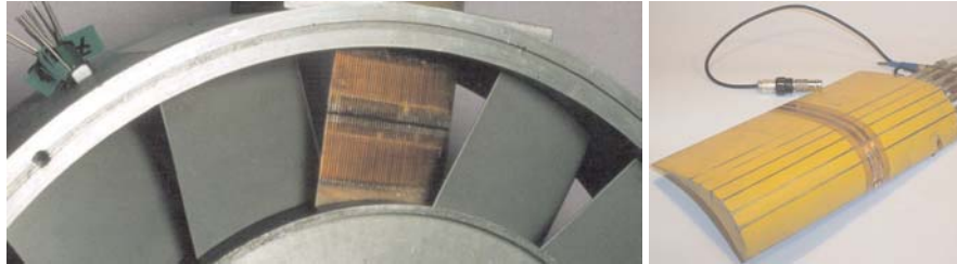
Figure 5. Turbine stator vanes with glue-on probes for boundary layer measurements
