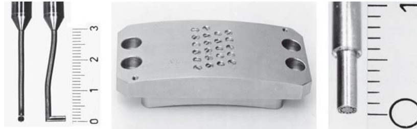
Figure 2. Single sensor dynamic pressure probe (left), dynamic pressure transducer at the casing (center and right)
