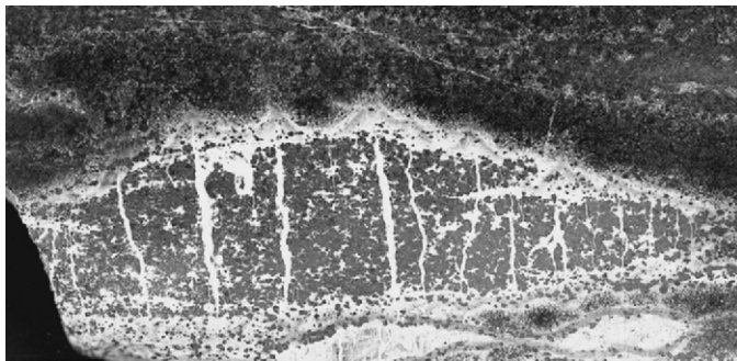
Figure 1. Hand specimen of olivine rock (dunite) near Orhaneli/Turkey, showing magnesite veinlets inside a chromite lens, topped with serpentine where the veinlets pinch out into the surrounding dunite. [Please see this figure in the color section at p. 309]
