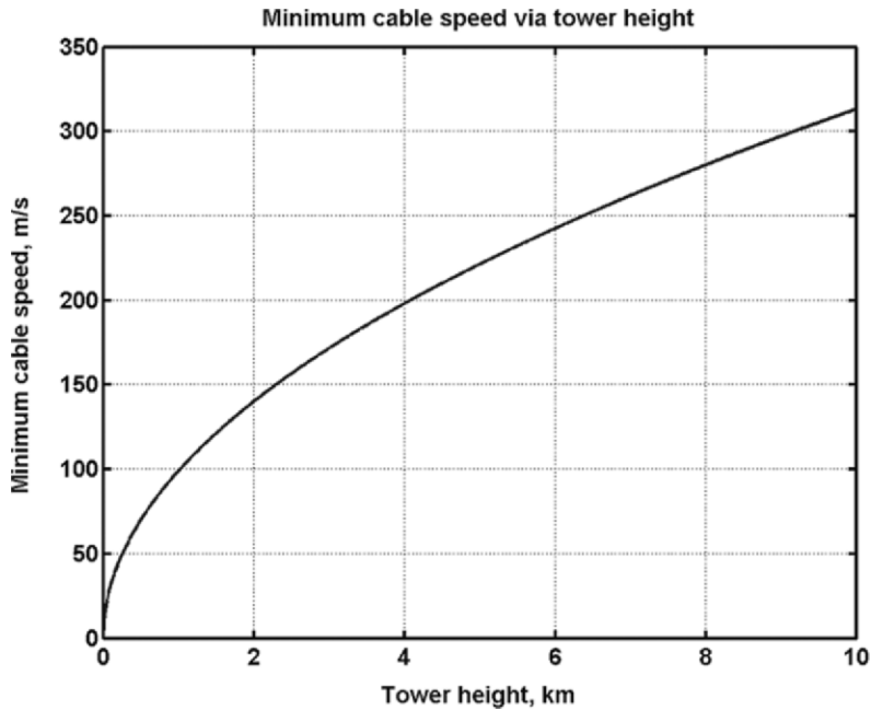
Figure 10. Minimum cable speed versus tower height
