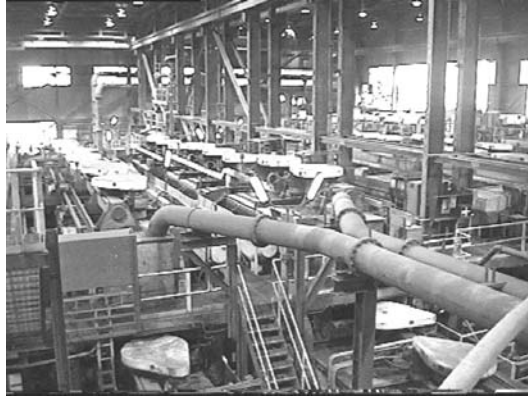
Figure 20-8. The flotation hall. Flotation means, the slurry of milled ore and water is foamed with air. Bubbles are adsorbed to ore particles so that they rise from the slurry. To enhance efficiency, chemicals are added, mainly lime.
