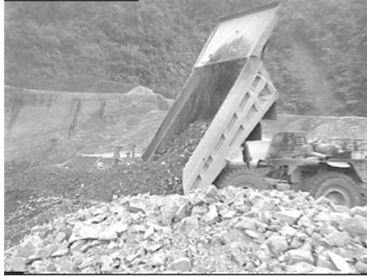
Figure 20-5. Dead rock and ore is removed by giant trucks, which haul 150 tons in a load.
