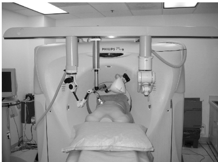
Figure 10-4. Three navigation tools integrated with the Brilliance 16 CT at the NIH Clinical Center. Left: Passive position-sensing arm tracking a US-HIFU assembly. Center): Electromagnetic generator for instrument-tip tracking. Right: Six-axis robot with laser end-effector. The retractable CT gantry frame registers diagnostic and therapeutic devices in multiple (detent) positions and in the CT's coordinate system, and facilitates their easy deployment.
