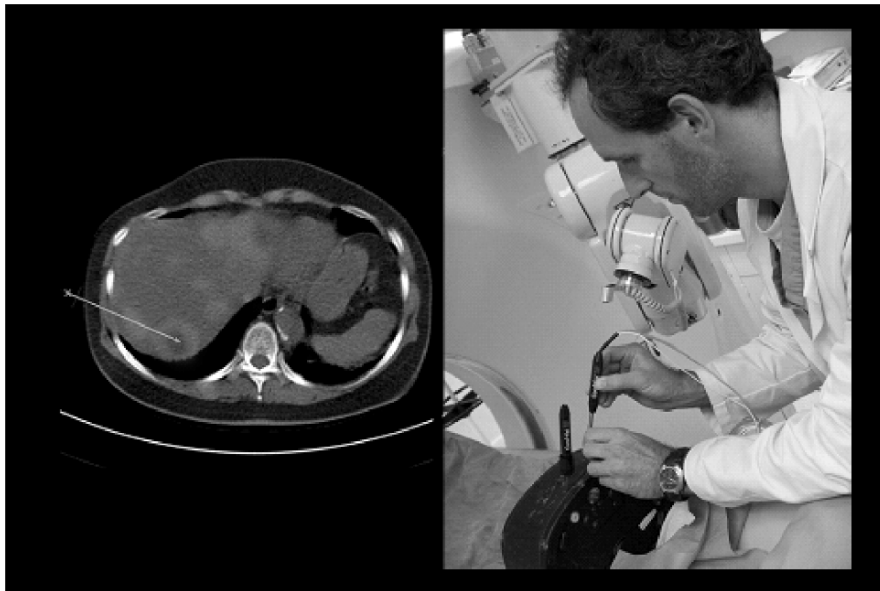
Figure 10-3. Left: F^{18}DG PET-CT data set used with point-and-click GUI to plan trajectories for CT Guided robot. Right: Dr. Wood uses laser guidance to place a Radionics triple-cluster RFA electrode in a CIRS Model 57 (CIRS Norfolk, VA) abdominal phantom.
