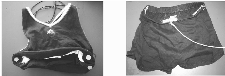
Figure 1-6. Underwear provided with sensors (Philips Research).
