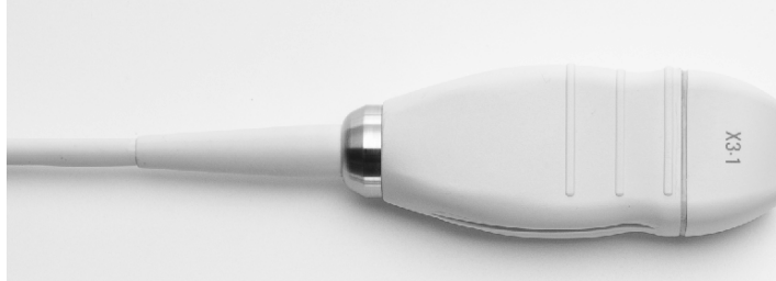
Figure 7-1. A two-dimensional array (X3-1 Philips) for real-time four-dimensional cardiac imaging.
