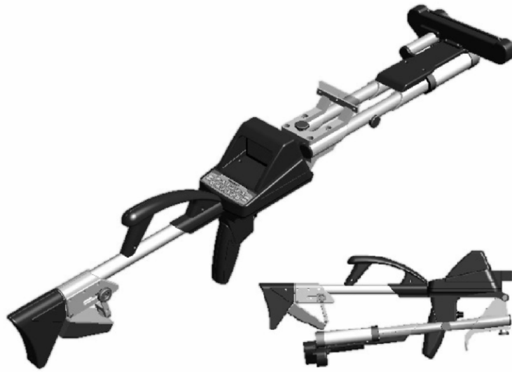
Figure 21.4 The third laser relascope prototype, opened out for measuring and folded for carrying.
