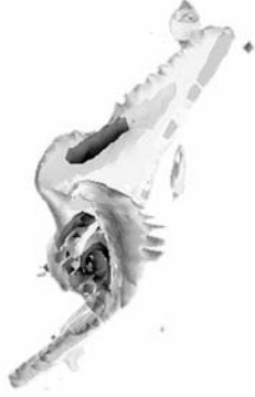
Figure 1. Isosurfaces of the [-(S_{ik}\Omega_{kj} + S_{jk}\Omega_{ki})]_+ eigenvalue (plotted using the white color), and Q (black), obtained from DNS.
