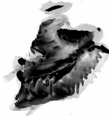
Figure 2. Front view of isosurfaces of [-(S_{ik}\Omega_{kj} + S_{jk}\Omega_{ki})]_+ (white), Q (black), and the dissipation term (dark gray).
