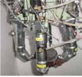
Figure 23. Slave hand as a powerful hydraulic four-finger robot hand.
