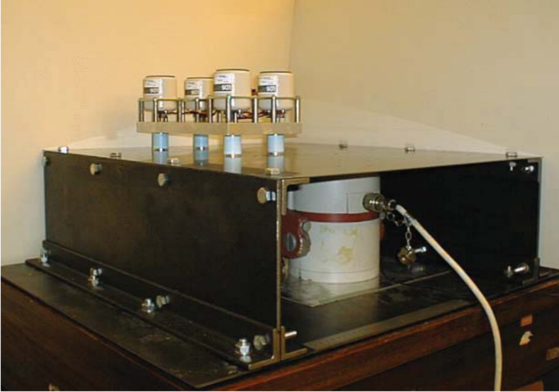
Figure 3. Experimental arrangement of 4 active mounts isolating the equipment structure from the vibration of the buss structure.
