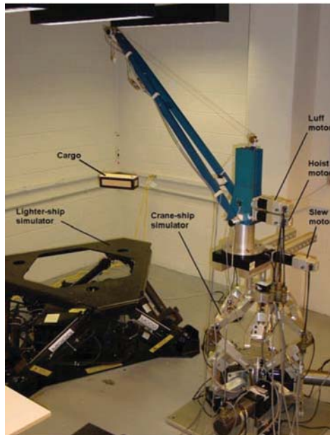
Figure 11. A 1/24 scale model of the T-ACS crane mounted on a three-degrees-of-freedom platform.
