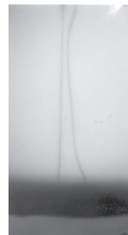
Figure 9: Experiments: Re_{inlet} = 1500 , v_2 = 680v_1 ; right dye streak indicates the spread of momentum into the ambient, whereas the jet fluid is confined to a smaller region
