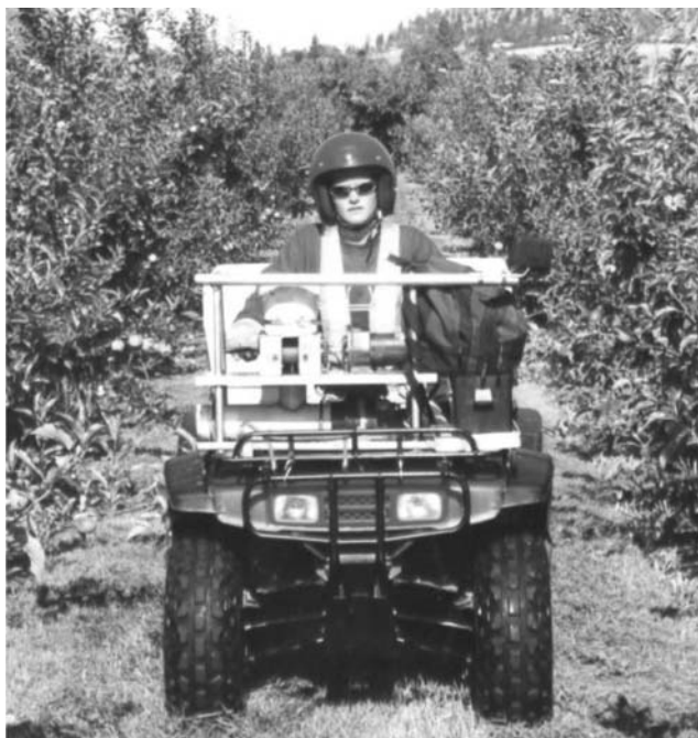
Figure 4. All-terrain vehicle (ATV) releasing chilled irradiated codling moths. (Photo from SIR Program (2004), reproduced with permission.)
