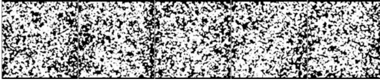
Figure 13.10. Five cuts through the porous filter cake, at different depths into the sample.
