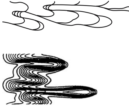
Figure 8.2. Tip splitting (top) and shielding (bottom) in viscous fingering
