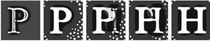
Figure 3. Reconfigurable assembly. Initially, the electrode voltage pattern is the letter P, and the adsorbates assemble accordingly. Then switch the electrode voltage pattern to the letter H, and the adsorbates re-assemble. The electrode voltage is high, so that the electrode voltage pattern overwhelms the natural pattern of the adsorbates.
