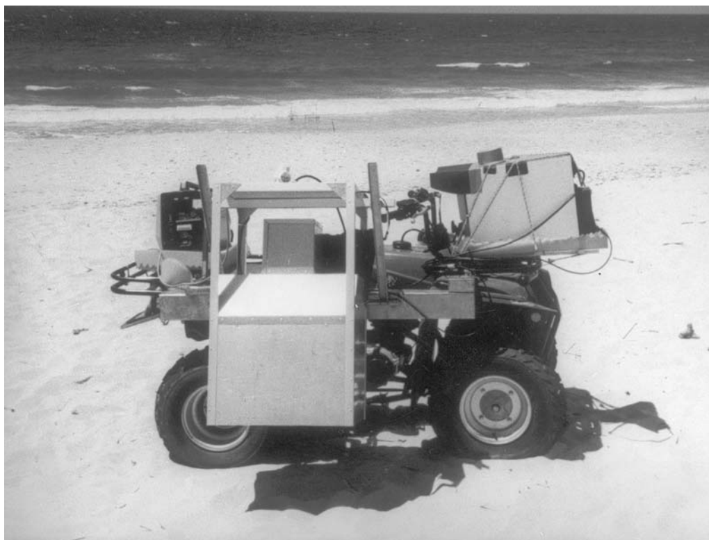
Figure T50 The SADAM system of Pinto et al. (1994) for in situ mapping of surface dispersal of fluorescent grains. It consists of an ATV, a dark camera with UV light, and computer with image processing software.
