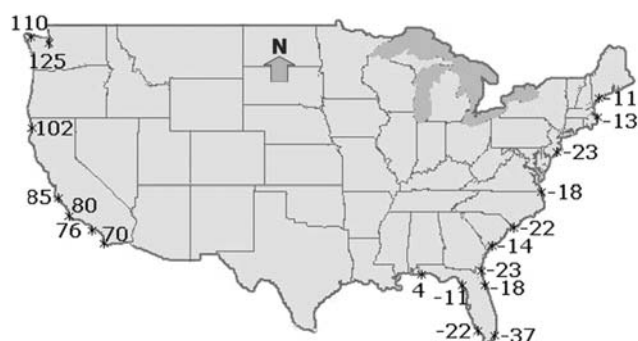
Figure T13 Height in centimeters of MSL datum above NAVD88 (redrawn from USACE, 2002).
