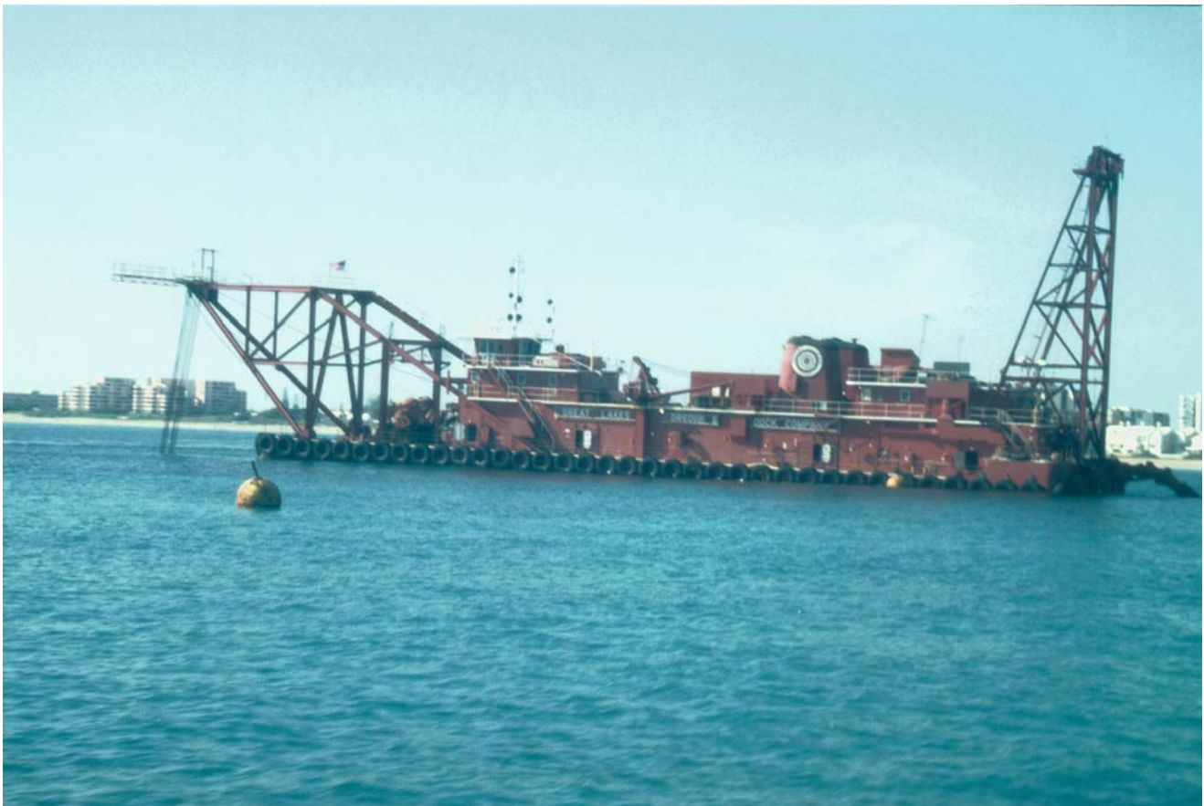
Figure B27 Large ocean-going dredge operating off the coast of southeast Florida. The Illinois , owned and operated by the Great Lakes Dock and Dredge Company (Oak Brook, IL, USA), is one of the largest suction cutterhead dredges in the United States. The 98-m long dredge, which digs to a nominal depth of 32 m, has a 760 mm discharge diameter and can pump sand 7,635 m without booster pumps. With total installed power of 8,400 kW, and 1,400 kW cutter power coupled with 662,000 L fuel capacity, the Illinois is ideal for working offshore for long periods in rough weather conditions. The dredge is not self-propelled and must be moved to projects by tugboats. When on site, the dredge has a large swing radius using a system of anchors and cables to maneuver within about a 300 m range without resetting the anchors. This dredge can work in swell up to 2 m high and usually operates 24 h a day when possible. Beach-quality sand from the borrow area is pumped in a pipeline to the beach. Because the dredge might operate up to 2 km offshore, the pipeline is floated on the surface near the dredge for ease of maneuverability and submerged near the shore for safety of boaters and beach users.
