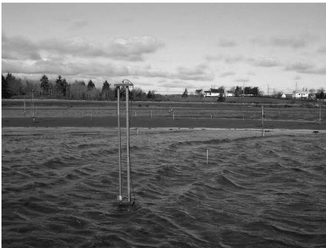
Figure B13 Resistance wave staffs (left) deployed over an intertidal ridge and runnel, Nova Scotia, Canada. A grid of depth of disturbance rods is deployed across the bar (center) and frames supporting OBS and electromagnetic current meters can be seen in the far right.
