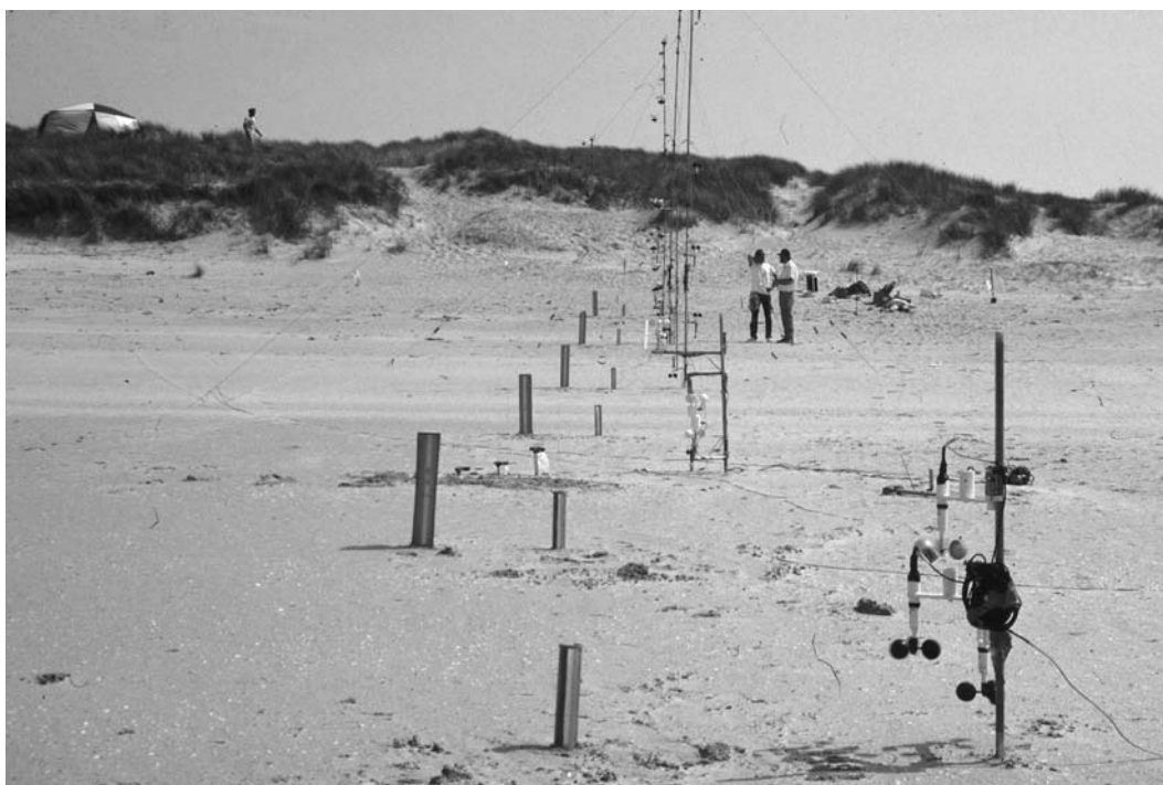
Figure B12 Array of cup anemometers and wind vanes mounted on towers to measure wind flow over the beach foreshore at Innisfree Beach, Ireland. Two versions of integrating sediment traps are seen on the left—the smaller traps are cylindrical traps after Leatherman (1978) and the other traps are wedge traps (Nickling and McKenna-Neuman, 1997).
