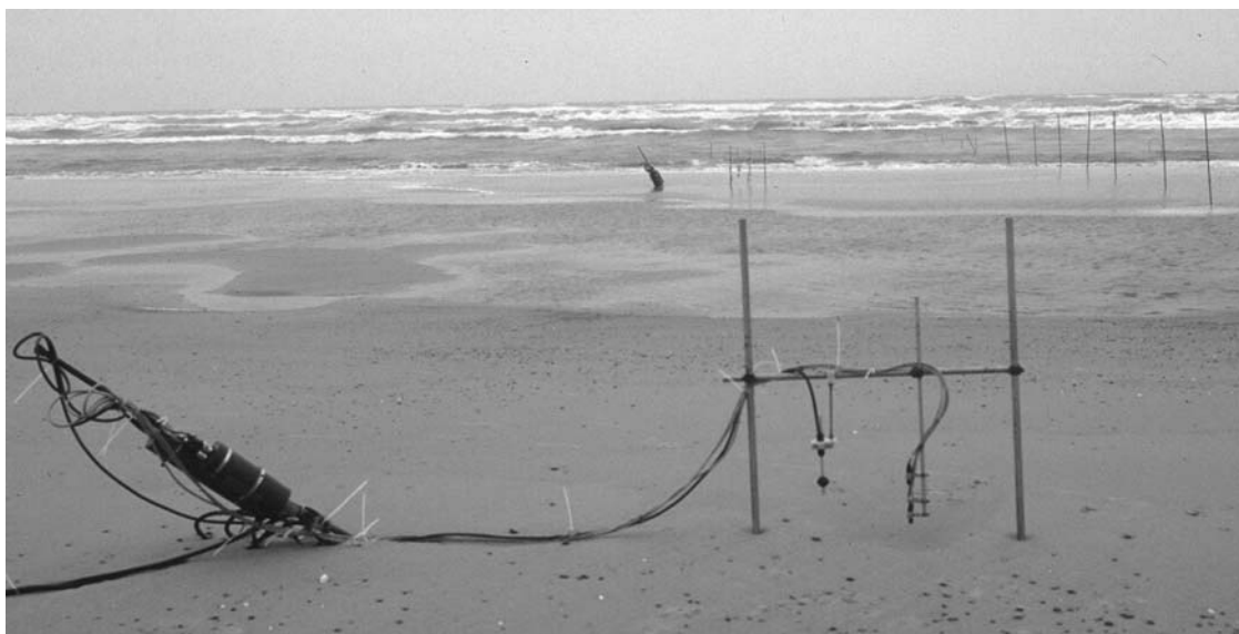
Figure B14 Electromagnetic current meter (left) and three OBS probes mounted on a “goalpost” in the intertidal zone, Skallingen, Denmark. Electronics for the current meter are installed in the waterproof housing secured to a pole jettied into the sand to the left of the goalpost. A profile line of large depth of disturbance rods is visible at the right.
