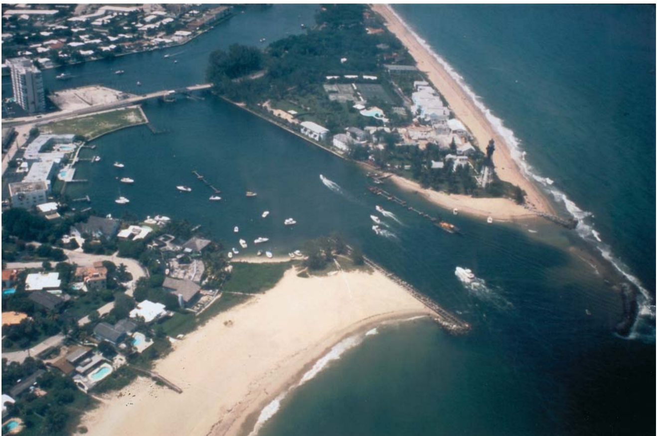
Figure B26 Hillsboro Inlet, Broward County, southeast Florida. Erosion of the downdrift coast, seen in the coastal offset (photo center), was caused by stabilization of this inlet by jetties. Subsequent construction of a weir jetty on the updrift side of the inlet permitted sand to overwash into an interior sand trap on the landward side of the jetty. A floating dredge sucks the sand from the trap and pumps it to the downdrift side of the inlet via a submerged pipeline. Dredging is mostly conducted during storms when sediment is overwashed through the weir because the trap quickly fills with sediment. If the sand trap is not cleared as it fills, excess sediment spills into the navigation channel where it becomes a hazard to boaters. This sand bypassing arrangement moves 100% of the estimated net littoral drift to the downdrift beach which is thus maintained in a healthy state.
