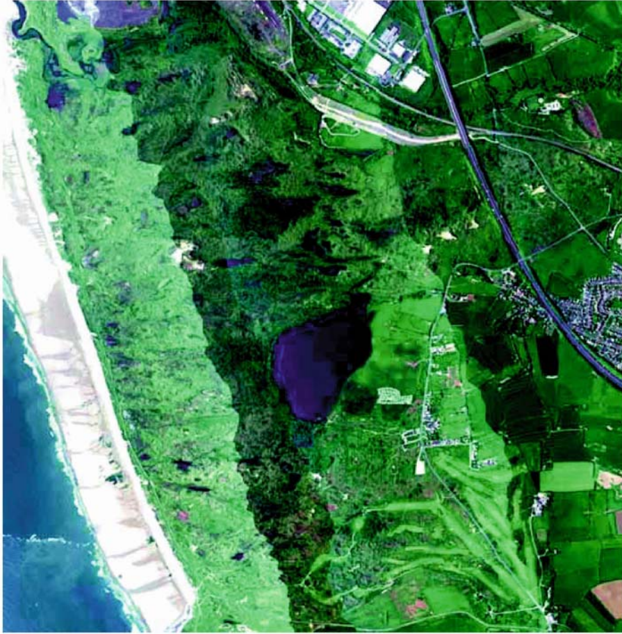
Figure 31-1. In this image, generated in ENVI 1 , we can see across-track radiance trends within each flight strip. These made it impossible to classify the habitats in the mosaicked CASI image. The major problem was that there were differences in the radiance values within the flight strips as well as between them. This artefact of the data collection process is most visible in the flight strip containing Kenfig Pool, which is bright green along its eastern edge but a paler green along the western edge.
