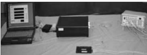
(a) Practical devices for monitoring system based on FBG sensors
