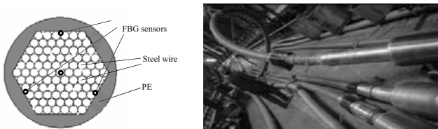
Figure 6 Smart cables based on FBGs
