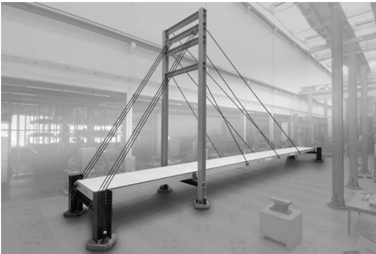
Figure 1. Cable stayed footbridge in the Empa-laboratory.
