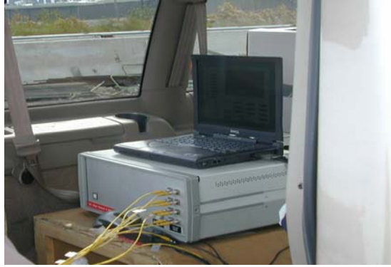
Figure 3 Example of a mobile long gauge sensor interrogation unit during monitoring of the cracks in a bridge deck
