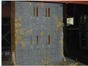
Fig. 7 Structural model of reinforced concrete bridge pier
