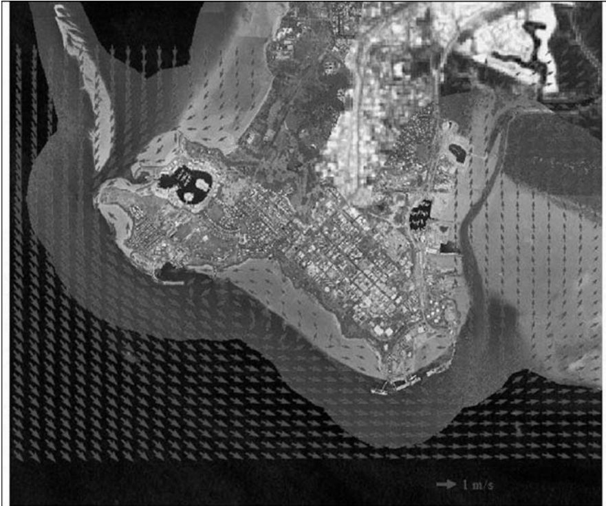
Figure 4. A snapshot of the predicted distribution of the horizontal currents at flood tide near Darwin City during a spring tide. The blue shading indicates the intertidal area.
