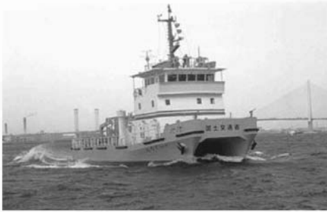
Figure 6. The marine environmental improvement vessel to collect floating garbage in daily operational basis in Tokyo Bay.
