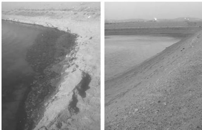
Figure 9. Details from the “Halliburton Pit”: tar floating on the water surface some six weeks after filling and inoculation (left) and the clean banks after ca six months (right).
