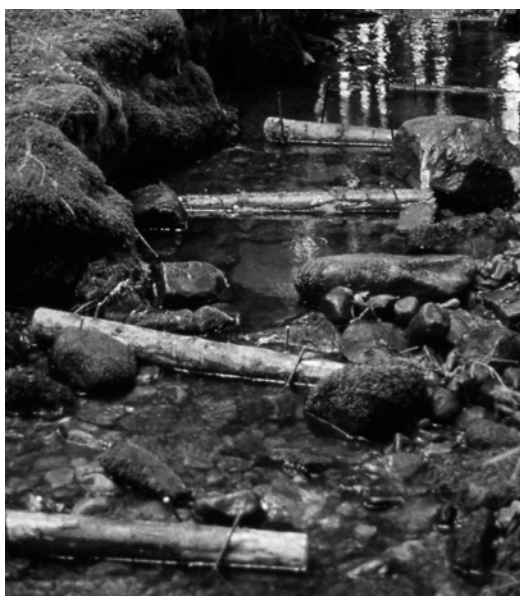
Figure 3.2. Use of wooden logs as litter traps, as used by Pretty & Dobson (2000). Note that each piece of wood is held in place by four steel poles, arranged in pairs upstream and downstream and each bent over the log at the top to stop it from being entrained by high water flows. Photo M. Dobson.
