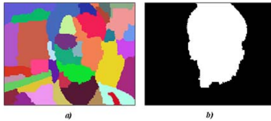
Figure 12. a) Sector of the human skins in the (U, V) plane; b) Threshold of Fig. 11a according to the skins sector.
