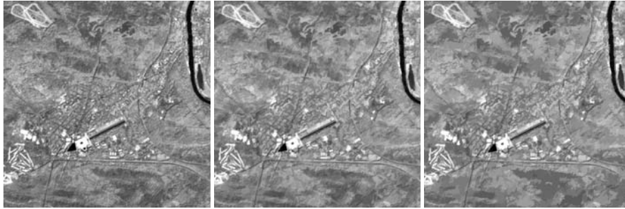
Figure 5. Left: Landsat panchromatic image of Fontainebleau (12.5m resolution), 481 \times 481 pixels (122,582 0-flat regions). Middle: Output of iterative seeded region growing up to a size of 25 pixels (4,071 0-flat regions). Right: After MCISRG merging using the optimum contrast threshold value of 4 grey levels (2,399 0-flat regions).
