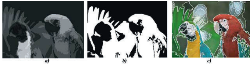
Figure 10. a) Segmentation of the saturation (presented in grey tones); b) optimal threshold of a); c) final synthetic partition, superimposed to the initial image.
