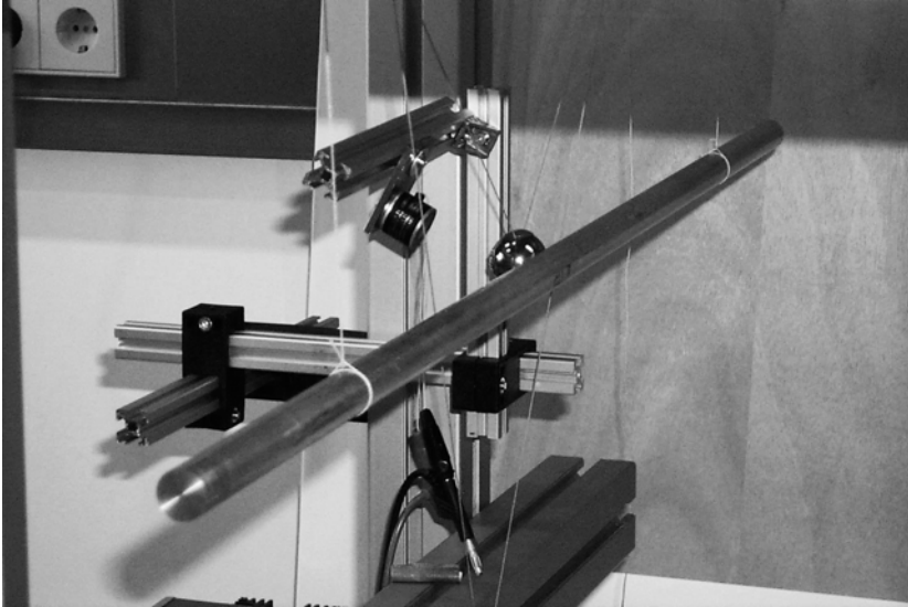
Fig. 9. Experimental setup with the impact on the beam
