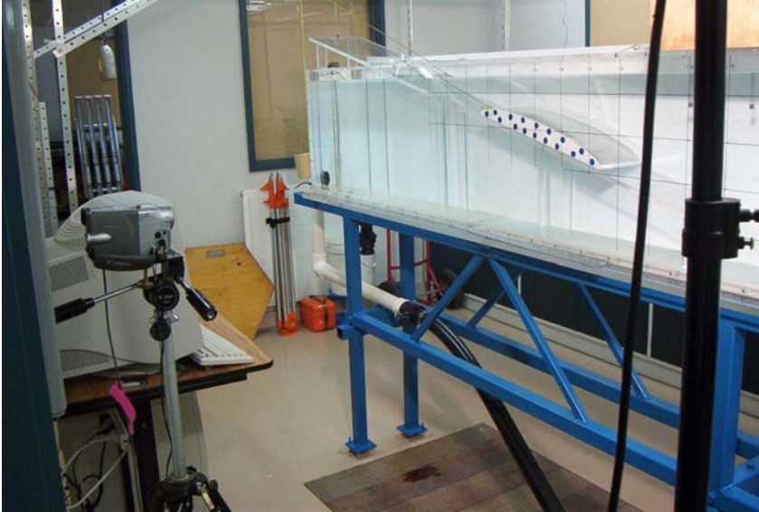
Fig. 1. Photograph of experimental apparatus for Phase 1 of the experiments using a semi-elliptical solid block as the landslide.
