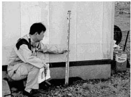
Fig. 5. Photos of a) tsunami deposits on the quay of the Tokachi harbor and b) the water line on the building in the Tokachi harbor.
