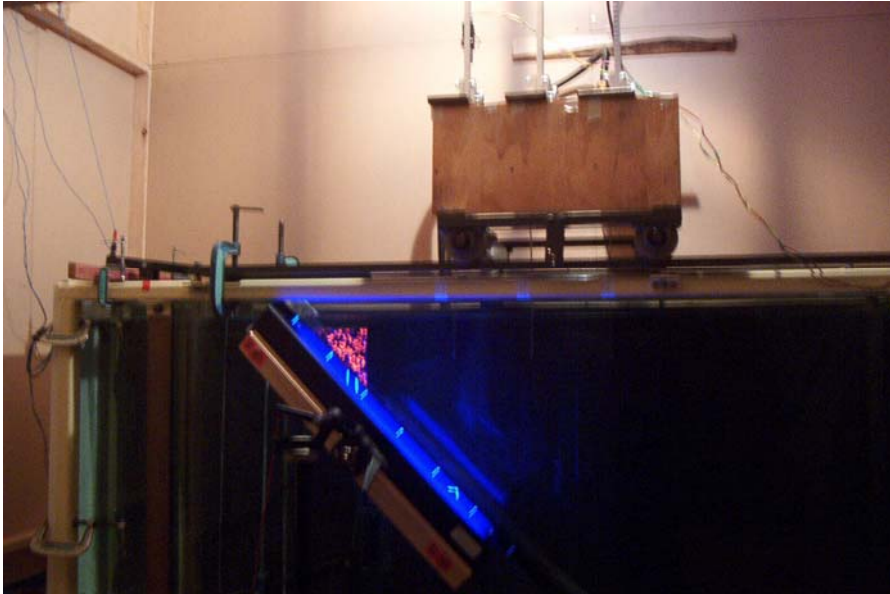
Fig. 3. Photograph of experimental set up for the second phase of experiments using triangular solid block slides as well as granular material slides.
