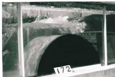
Figure 6: Example wave transmission over a submerged semi-cylinder breakwater
