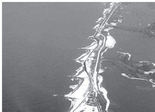
Figure 14: Lee Erosions Past Groynes and Breakwaters
