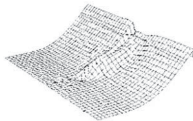
Figure 6: Long-shore variations of wave set-up around a submerged groins
