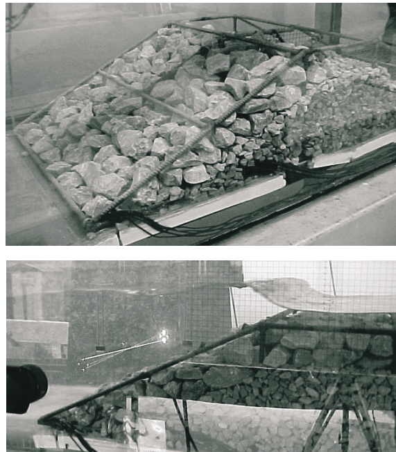
Figure 15: The DELOS Project flow tests. Construction of the “short-crested” (0.25 m) structure and LDA measurements during the tests
