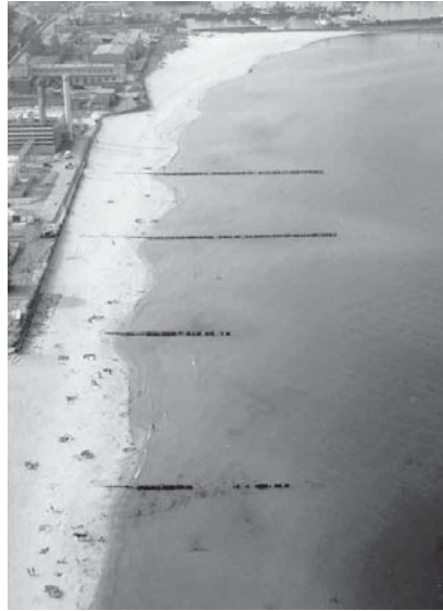
Figure 8: Combined effect of groin field and artificial beach fill, lee side, Władysławowo harbor (Poland)
