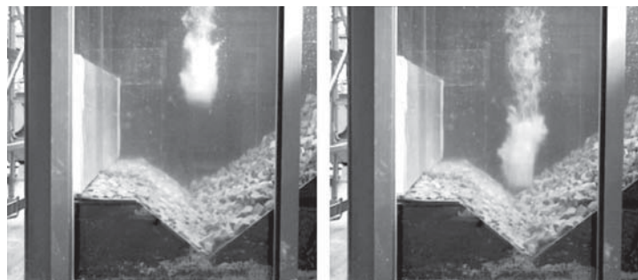
Figure 4: Dropping of a block in the laboratory (Verhagen et al., 2002)
