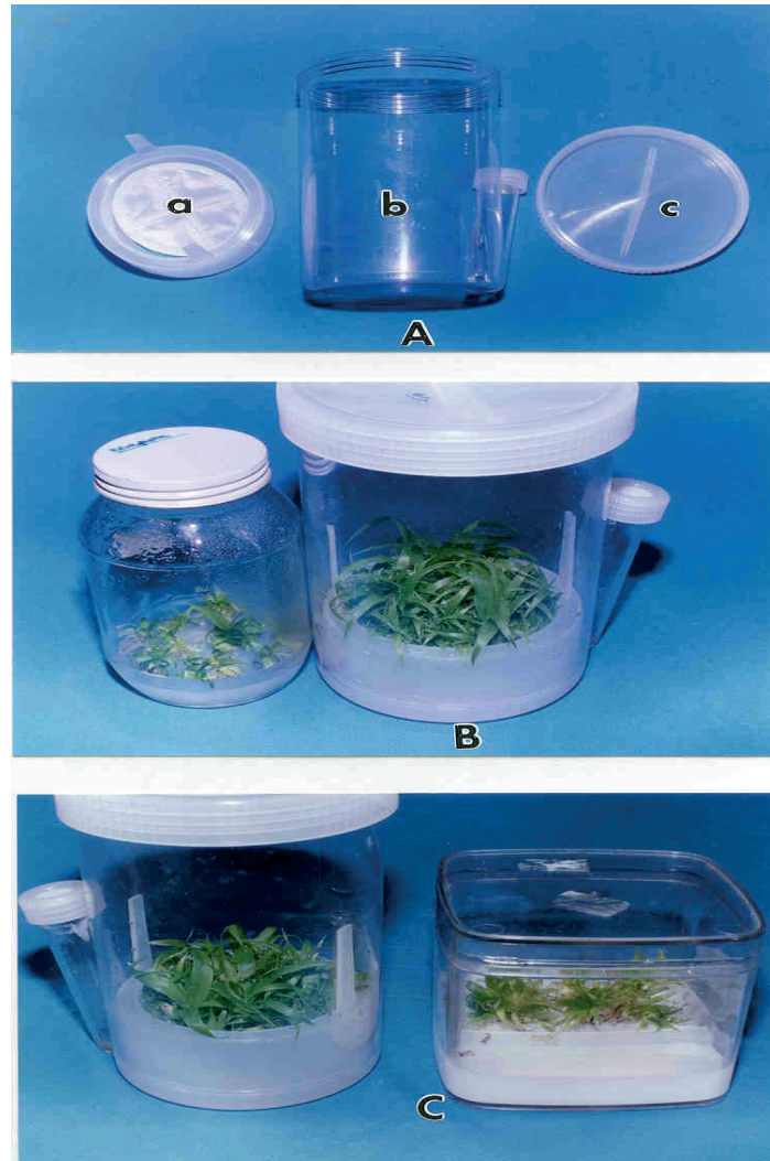
Figure 1: (A): Growtek bioreactor with floating explant-holder (a) main vessel with side tube (b) inside of the lid (c) shown separately; (B): pineapple shoot cluster production in glass jars and Growtek; (C): pineapple shoot cluster propagation in Life Guard and Growtek.
