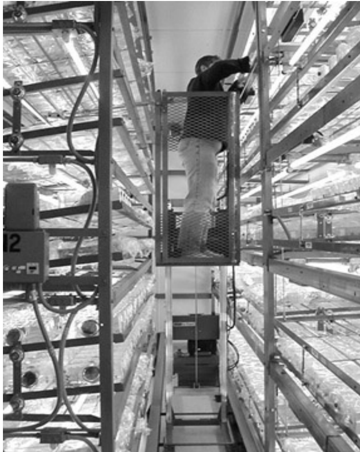
Figure 6: Thin film rocker system scaled-up for efficient space utilization in culture room.
