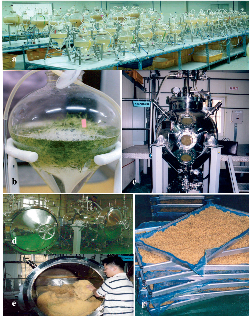
Figure 3: (a) Bioreactor culture (5-litre sized BTBB) of adventitious roots of ginseng ( Panax ginseng C.A. Meyer); (b) Mass propagation of Sibirian ginseng somatic embryos in 5-litre BTBB from embryogenic cells; (c) Pilot scale BTBB (500-litre); (d) Pilot scale column type bioreactor (1000-litre); (e) Harvesting of adventitious roots from 500-litre BTBB eight weeks after inoculation; (f) Harvesting of Sibirian ginseng somatic embryos from 500-litre BTBB after 30 days of culture
