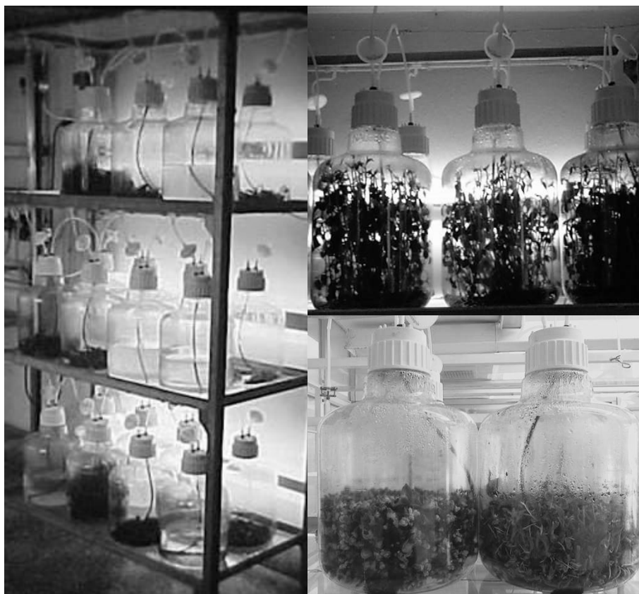
Figure 1: Production facility at the Institute of Plant Biotechnology, Cuba (left). Potato microtuber production (up right), and banana propagation in 10-litre twin flask TIS (low right).
