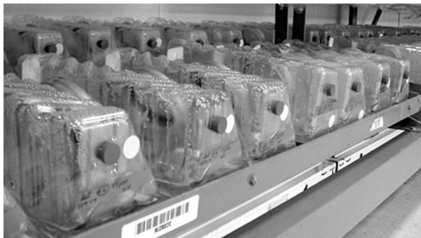
Figure 2: Rectangular vessels facilitated a slow moving wave of media to migrate the length of the vessel with the motion of the shelf.
