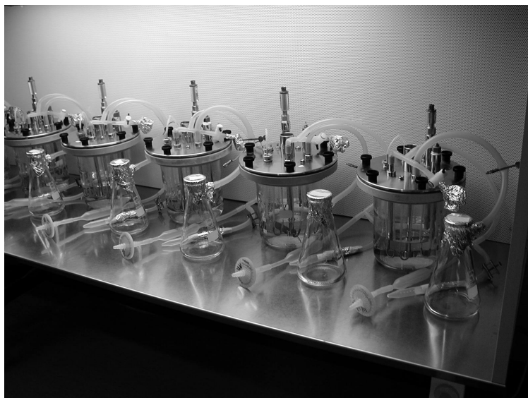
Figure 2: Bioreactors after autoclaving, cooling off in the laminar flow hood before final assembly in an acrylic outer container thereby providing a water-jacket for temperature control.
