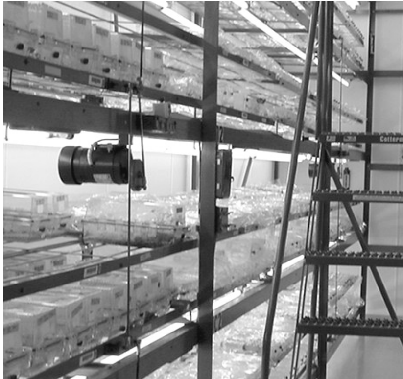
Figure 1: Agitated thin-film rocker system is a simple, temporary-immersion liquid culture.
