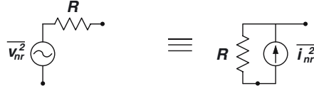
Figure 2.7: Noise voltage and noise current of an arbitrary resistor.
