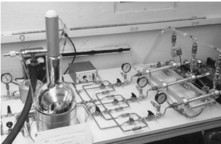
FIGURE 11.24. 1982 JPL breadboard hydride–hydrogen cryocooler (650 mW at 29 K).
