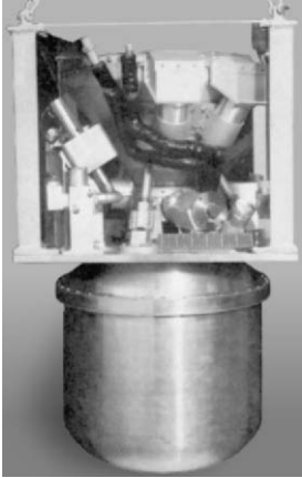
FIGURE 11.4. Lockheed solid carbon dioxide cryostat flown on SESP 72-2 in October 1972.
