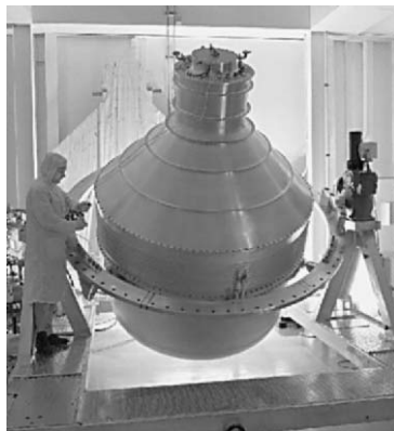
FIGURE 11.51. GPB superfluid helium dewar.
