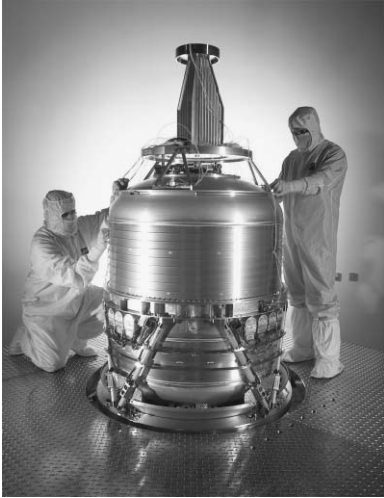
FIGURE 11.50. SIRTf superfluid helium dewar.
