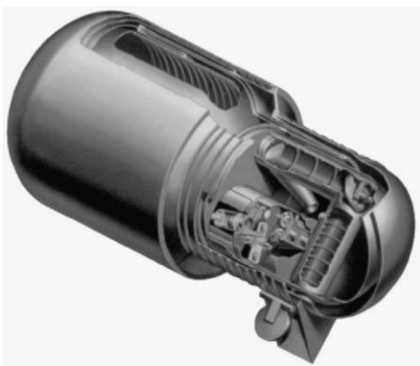
FIGURE 11.26. Two-stage solid neon-carbon dioxide dewar built by Lockheed for the CLAES instrument launched in 1991 on UARS.
