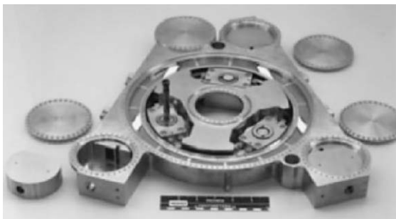
FIGURE 11.19. Hughes rotary magnetic cooler for cooling between 10 and 20 K.
