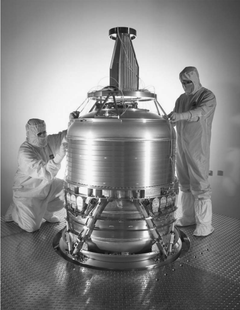
FIGURE 9.2. Spitzer space telescope cryogenic tank assembly being prepared for vibration testing (tank volume: 363 L) [16].
