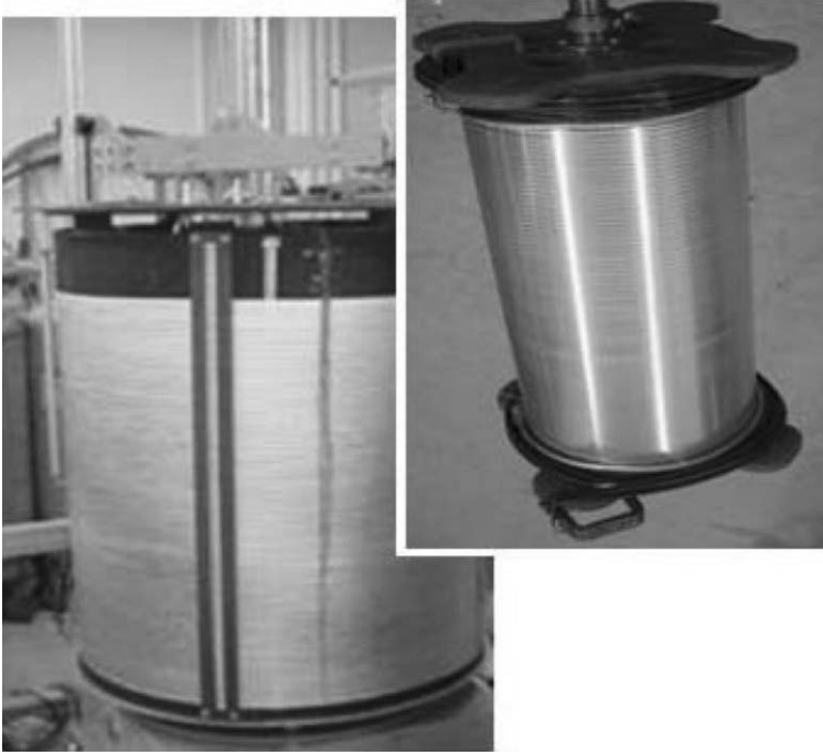
FIGURE 13.8. Coated conductor tapes produced by high-rate PLD on YSZ-buffered SS tapes (40 m, 235 A/cm-width) from EHTS (right [52]) and by multiplume PLD (212 m, 245 A/cm-width, Hastelloy/IBAD-Gd 2 Zr 2 O 7 /PLD-CeO 2 /multiplume PLD-YBCO) from SRL/ISTEC (left [54]).
