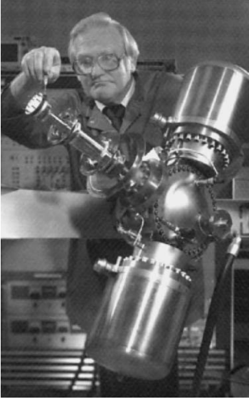
FIGURE 11.8. Hughes three-stage 12 K VM cooler used dual opposed pistons.
