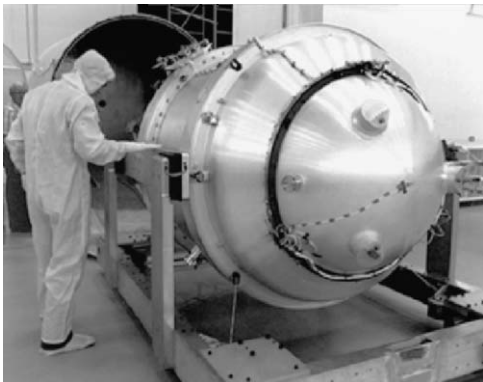
FIGURE 11.25. Ball Aerospace superfluid helium dewar used for COBE was derived from the IRAS dewar flown in 1983.
