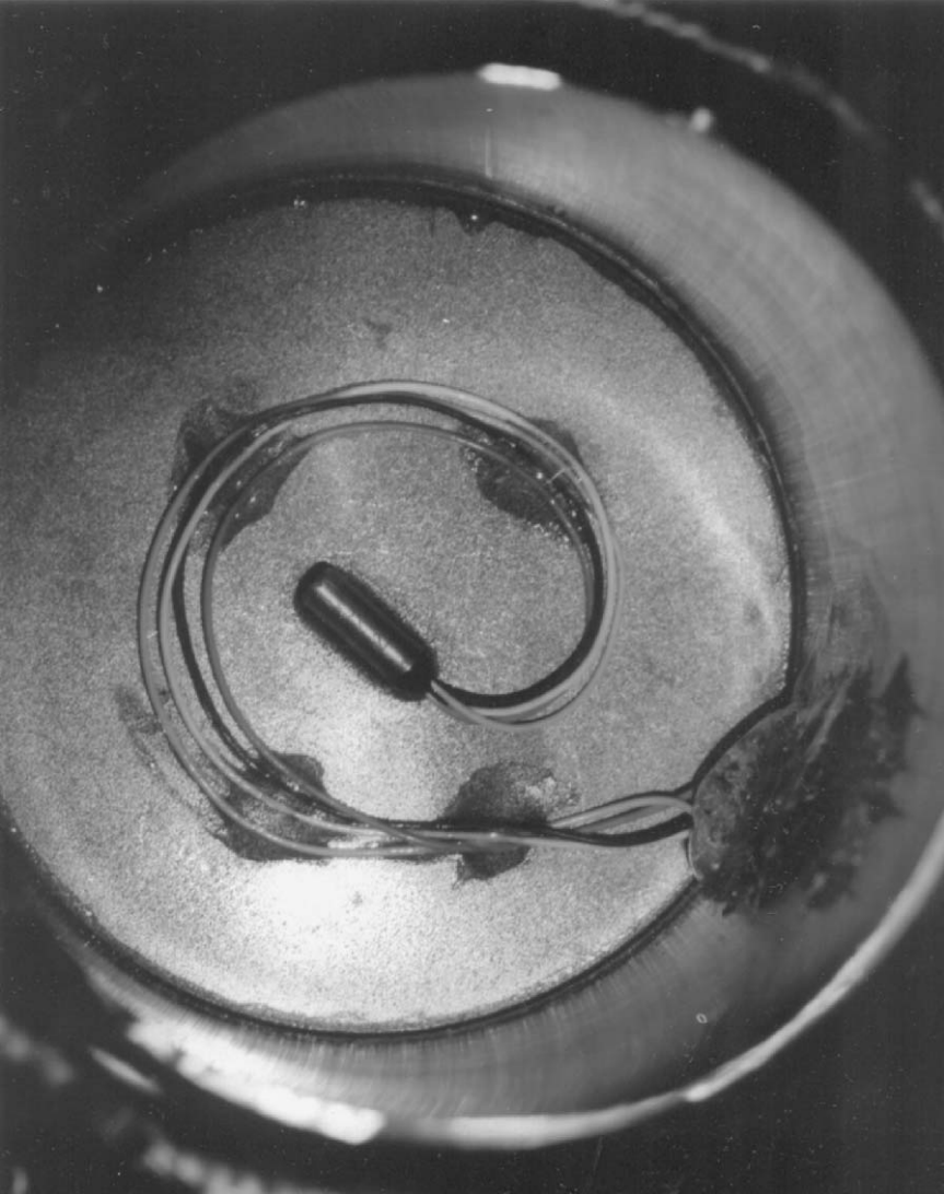
FIGURE 9.3. He II Phase separator for the IRAS SFHE tank. The plug is approximately 50 mm in diameter and manufactured by Mott Corporation (formerly Mott Metallurgical Corp.) from sintered nickel. The attached germanium thermometer is for determining the downstream helium temperature (from Ref. [20]).
