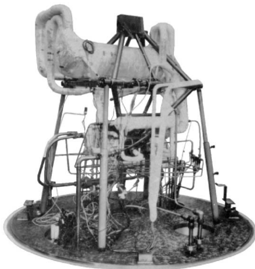
FIGURE 11.18. Garrett AiResearch turbo Brayton cooler.
