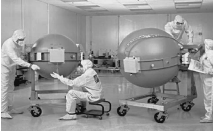
FIGURE 11.13. Over 60 of these PRSA dewars were built by Beech Aircraft and Ball Aerospace to supply the Shuttle's fuel cells with hydrogen and oxygen.
