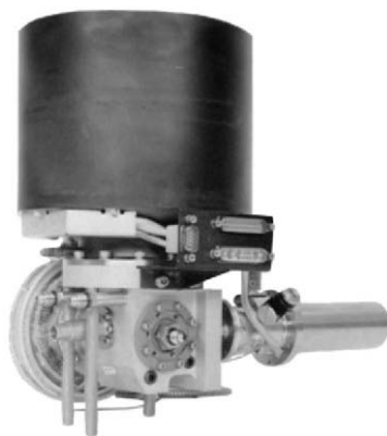
FIGURE 11.3. Hughes Aircraft two-stage VM cooler flown on SESP 71-2 in October 1971.
