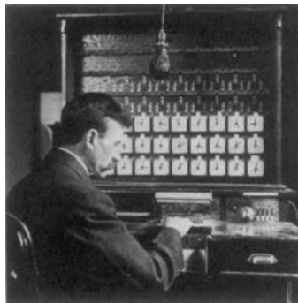
Figure 1.12. Tabulating machines. The Hollerith Tabulating Machine was an early data-processing system that performed automatic computation using punched cards. (Photograph courtesy of the Library of Congress.)
