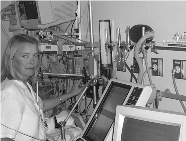
Figure 17.1. A nurse at a patient's ICU bedside. Above the nurse's head is the bedside monitor which measure and displays key physiological data, above her left hand is an IV pump connected to a Medical Information Bus (MIB), to her right are two screens of a patient ventilator and to the far right is a bedside computer terminal used for data entry and data review. ( Source: Courtesy of Dr. Reed M. Gardner)
