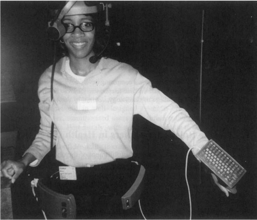
Figure 24.3. A wearable computer, including monacle display, voice input, belt-mounted central processing unit, and hand-mounted keypad. (Source: Photograph by Lawrence M. Fagan. Xybernaut, Mobile Assistant, and MA IV are registered trademarks of Xybernaut Corporation.)
