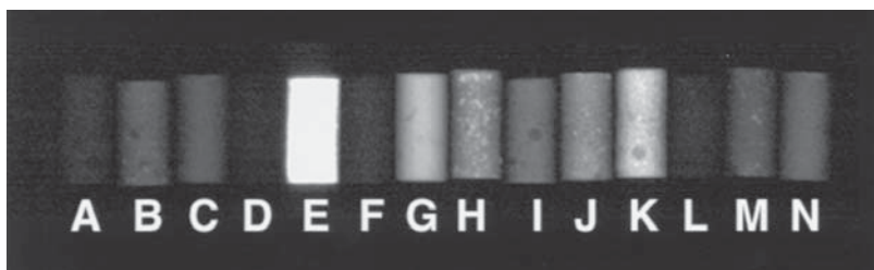
Figure 6.8. Radiopacities of various mixtures of cement: A, Simplex P; B, Simplex P with 20% by weight \text{BaSO}_4 ; C, Mathis recipe; D, Cranioplastic with 10 percent by weight \text{BaSO}_4 ; E, Fixos; F, Chemfix3; G, Orthocomp; H, Murphy recipe; I, Olan recipe; J, Simplex P with 30% by weight \text{BaSO}_4 ; K, Deramond recipe; L, Cranioplastic with 20% \text{BaSO}_4 ; M, Jensen recipe; N, Cranioplastic with 30% by weight \text{BaSO}_4 (see Jasper et al. [92] for composition details). (From J.M. Mathis, H. Deramond, and S.M. Belkoff [eds], Percutaneous Vertebroplasty . New York: Springer, 2002, with permission.)
