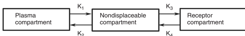
Figure 21.1. Schematic diagram of the compartmental model used to analyze PET and SPECT data in receptor imaging studies. K_1 , k_2 , k_3 , and k_4 represent the rate constants of the ligand movement between compartments.
