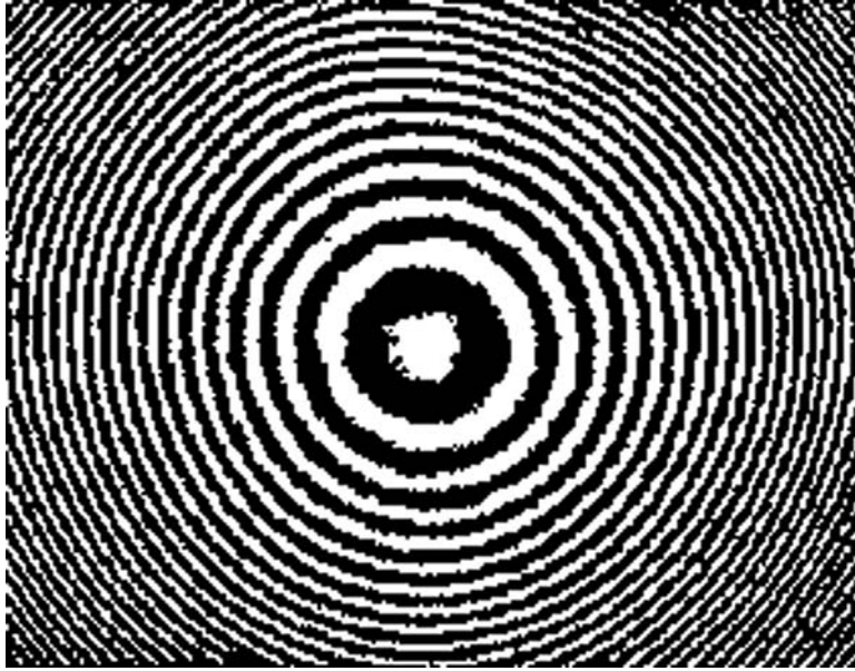
FIGURE 25.13. A typical interference fringe pattern obtained from the Si chip surface with the Twyman-Green interferometer.
