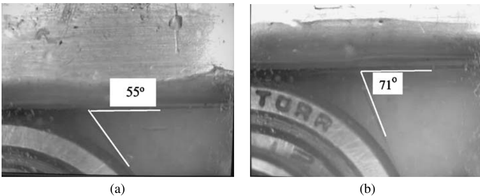
FIGURE 16.25. Measurement of peel angle: (a) dead weight is 0.83 N, (b) no dead weight.
