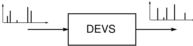
FIGURE 11.4. Input/output behavior of a DEVS model.
