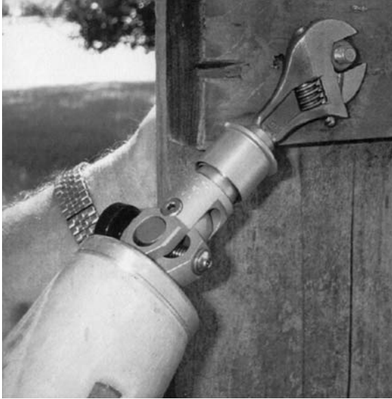
FIGURE 7.2. Modified hand tool for upper limb prosthetic user. Photo courtesy of Texas Assistive Devices, LLC, Brazoria, Texas.
