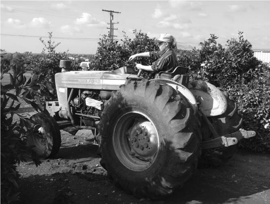
FIGURE 12.2. Driving equipment is one of the serious hazards for children on farms. This girl is driving a tractor without rollover protection. One concern is how much training she has received about operating the tractor and whether she would be able to respond to an emergency. Judgment can play a significant role in appropriate responses in emergency situations; many researchers have questioned which tasks are the age-appropriate for children working on farms. (Photograph by William Bennett, Jr.)
