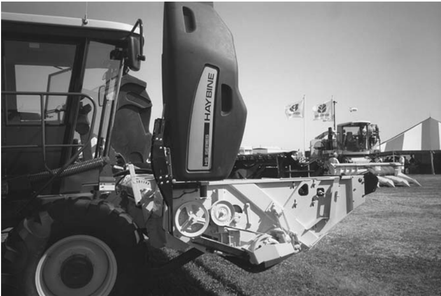
FIGURE 6.1. Hinged shield in raised (open) position for access.
