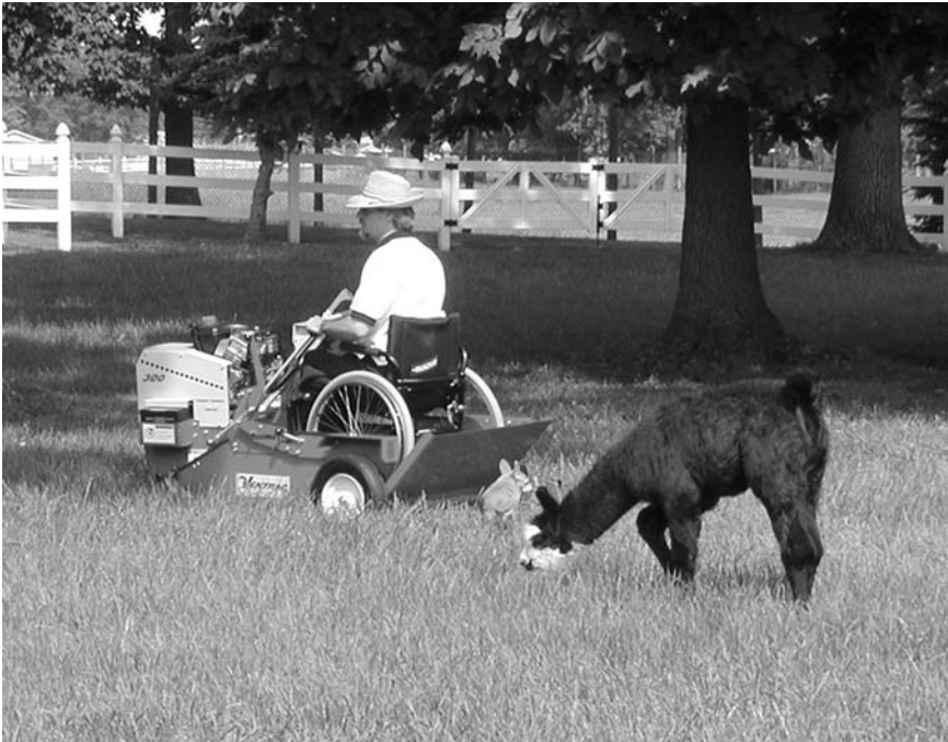
FIGURE 7.1. Ventrac-powered mobility aid for users of wheelchairs wanting access to rough terrain. Courtesy of Venture Products Inc., Orrville, Ohio.
