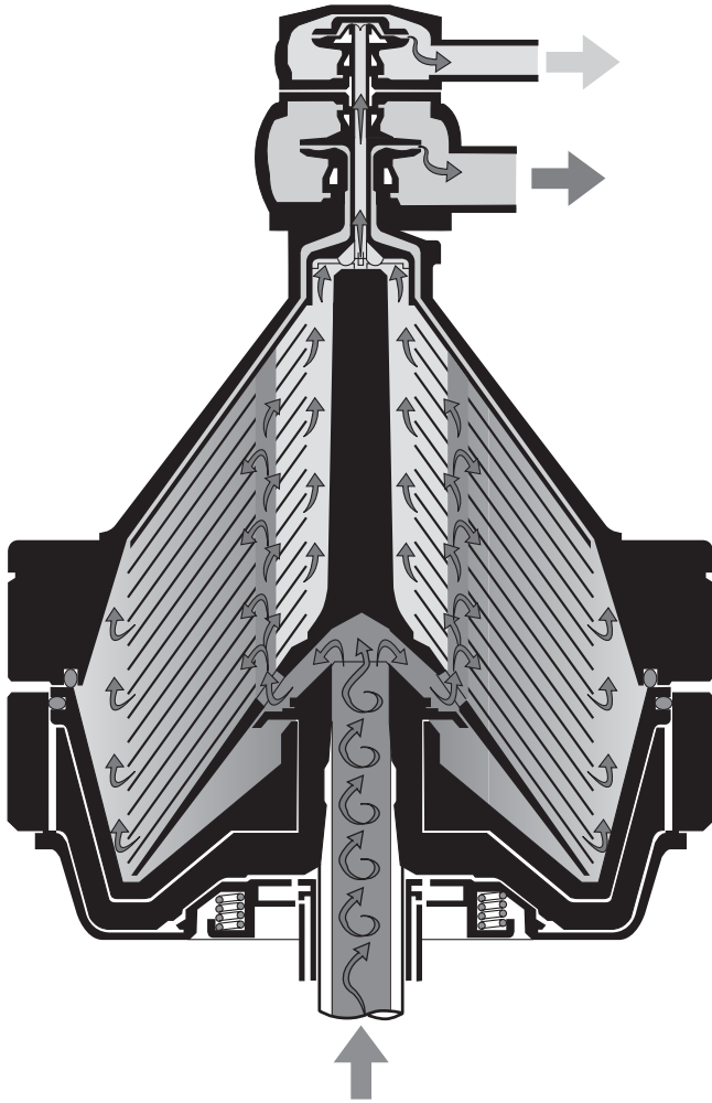
Figure. 5.2. Principle of operation of a centrifugal milk separator. Milk enters at the bottom of the unit and separates into heavier skim (dark grey) and lighter cream (pale grey) fractions which are recovered at the top of the separator (Reproduced with permission from Dairy Processing Handbook , Tetra Pak Processing Systems AB, Lund, Sweden, 1995).
