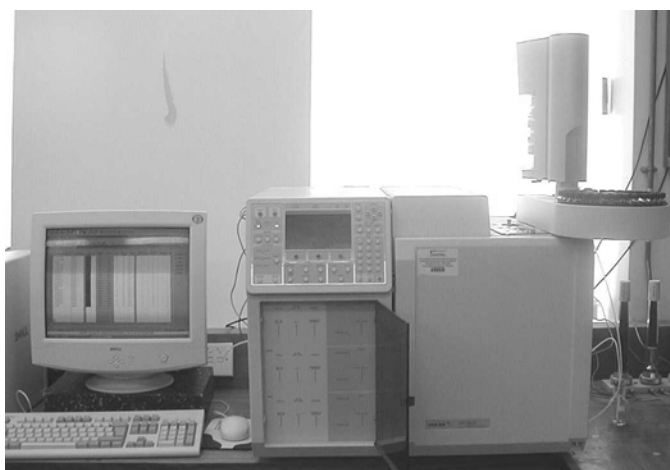
Figure 19.1. A Varian 3800 gas chromatograph coupled to a flame ionization detector and a Varian CP-8400 automatic injector operated by Varian Star Workstation Software Version 5.
