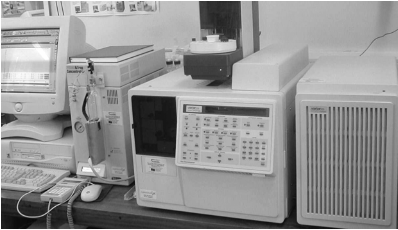
Figure 19.3. A Varian 3400 gas chromatograph with a Tekmar 3000 purge-and-trap concentrator and a Varian Saturn 2000 mass spectrometer detector operated by Varian Saturn GC/MS Workstation Software Version 5.41 k.
