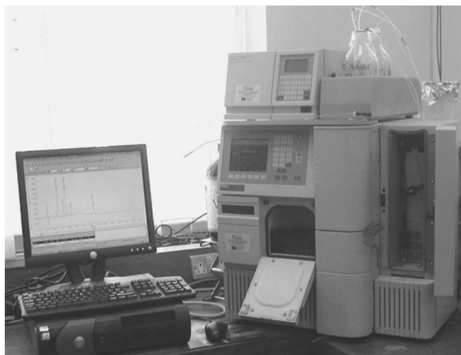
Figure 19.2. A Waters 2695 high performance liquid chromatograph with a Waters 2487 dual absorbance detector operated by Waters Empower Software.
