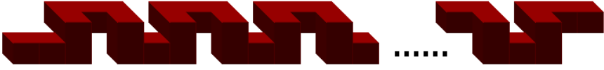
FIGURE 9.2. Schematic of a serpentine channel used in the experiments of (Liu et al., 2000).
