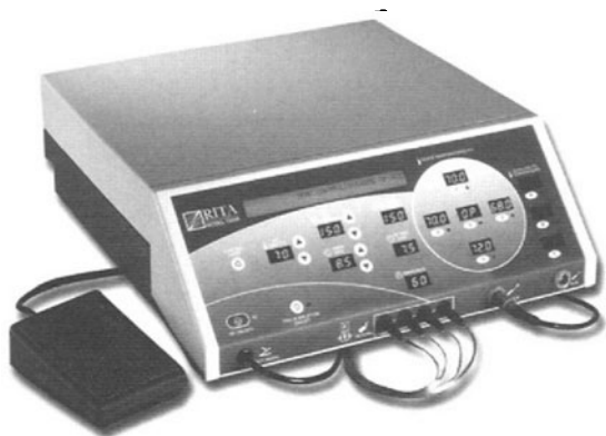
FIGURE 7.6. RITA Medical Systems, Inc. RF generator. The main control panel displays user-defined settings for the target tissue temperature, power, and time. Feedback to the user includes the actual RF power being delivered, the elapsed time, and tissue impedance. Up to eight thermocouple measurements to assess the temperature at the tines of the array (up to four) and at separate locations targeted with added needle-thermocouples can be displayed. In the figure, as an example, the device controls power to give average temperature readings of 70°C in four tines of an array. Temperature and time serve as the end points for ablation. (Photo courtesy of RITA Medical Systems, Inc.)
