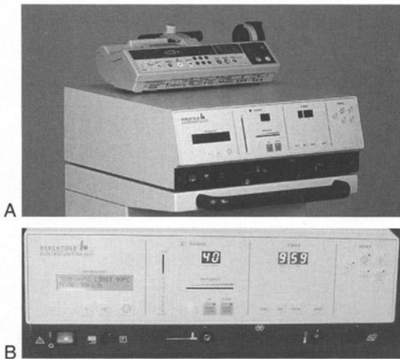
FIGURE 7.8. Berchtold GmbH & Co. RF generator and infusion pump. Saline is delivered to the RF electrode for infusion into tissue by the pump sitting atop the RF generator (A). The main control panel of the generator displays temperature, flow rate of the saline, power, and time (B). The system can be operated in either an impedance control or temperature control mode, whereby feedback to the user would be impedance in the tissue, or time and temperature, respectively. (Photos courtesy of Berchtold GmbH & Co.)
