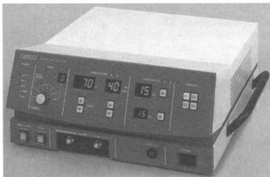
FIGURE 39.2. Microwave generator. Microwave generator is a surgical equipment originally developed in Japan to realize bloodless surgery particularly for fragile parenchymatous organs, like liver. Microwave generator emits a 2450-MHz microwave. In the treatment of liver tumors, not only percutaneous approach but also laparotomic and laparoscopic approaches are applied.
