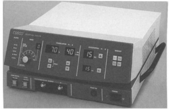
FIGURE 7.18. Alfresa Pharma Corp. microwave generator. The main control panel displays the user-selected parameters for the ablation. These include the output power, exposure duration, and the dissociation parameters mentioned in the text. Here, the ablation cycle is set for a duration of 40 seconds at 70 W with a dissociation current of 15 mA lasting 15 seconds. Also, the generator can power two probes simultaneously. (Photo printed with permission from Alfresa Pharma Corp.)
