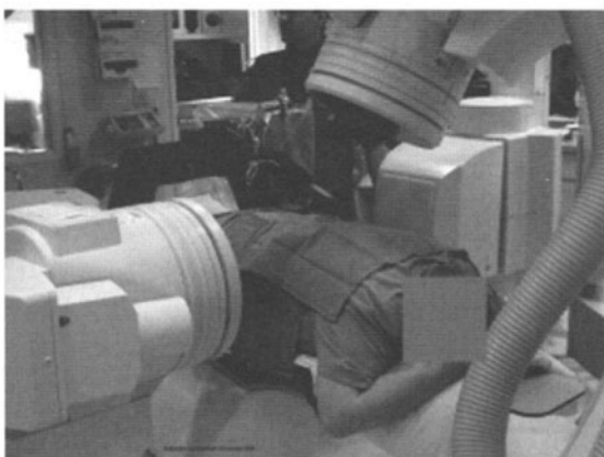
FIGURE 22.3. Table-mounted robot integrated with biplane fluoroscopy. Needle is driven using joystick controlled by physician. (Courtesy of Kevin Cleary, PhD, Georgetown University.)
