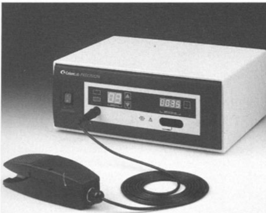
FIGURE 7.10. Celon AG Medical Instruments RF generator. The main control panel displays the power output by the device and the elapsed time. It operates in an impedance control mode. An audible tone provides the user with an indication that the tissue impedance has markedly increased, indicating complete ablation around the tip. (Photo printed with permission from Celon AG Medical Instruments.)
