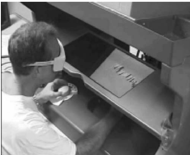
Figure 20.9. The Haptic Workbench incorporates a 3D visual display with the Phantom force-feedback device [14]. This device allows the user to feel attributes such as price momentum on a stock market chart [19].
