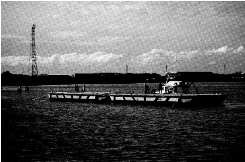
Figure 1.2. The shipwreck of the former whaler Day Dawn (1888) was lifted and moved using a barge, to protect it from being damaged during a Royal Australian Navy harbour redevelopment (photo courtesy of the Department of Maritime Archaeology, WA Maritime Museum).
