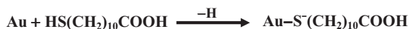
FIGURE 7.5. Thiolate formation with gold substrates: thiols react with gold surfaces by the formation of thiolates, which occurs with hydrogen loss by the sulfur atom.
