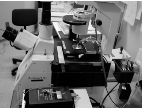
FIGURE 13.3. Schematic representation of the optical path through an inverted microscope (top). The MEA chip with the perfusion chamber containing the retina is placed on the microscope stage (middle). View on the recording setup (bottom).
