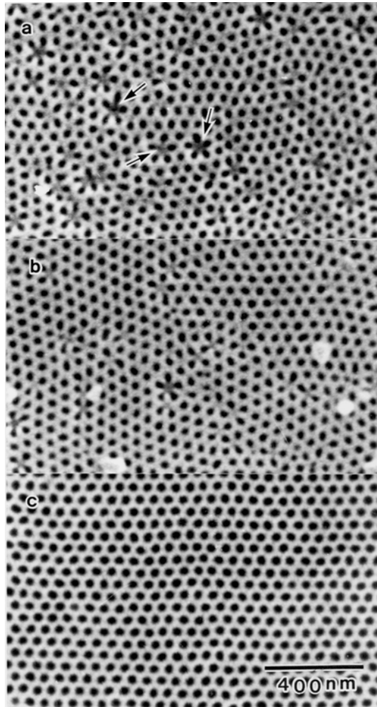
FIGURE 3.3. Dependence of the ordering of the hole arrangement of anodic porous alumina on the anodizing period in 0.5 M sulfuric acid solution at 25 V: (a) 9 minutes, (b) 36 minutes and (c) 710 minutes.
