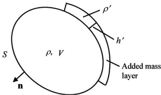
Figure 4.12-1. A crystal with a thin layer of additional mass on part of its surface.
