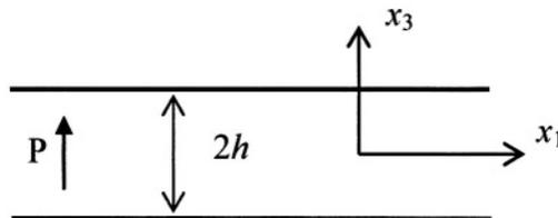
Figure 4.1-1. An electroded ceramic plate with thickness poling.
