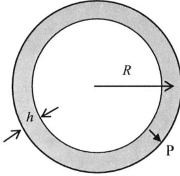
Figure 4.11-1. A spherical ceramic shell with radial poling.
