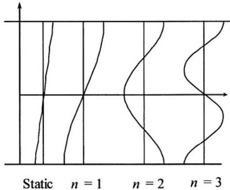
Figure 4.3-2. Thickness-shear deformation and modes in a plate.
