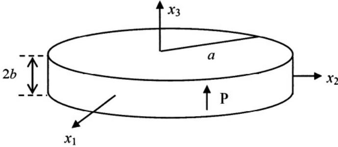
Figure 4.9-1. A circular ceramic plate with thickness poling.
