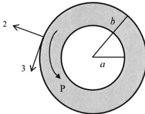
Figure 4.4-1. A circular cylinder with tangential poling.
