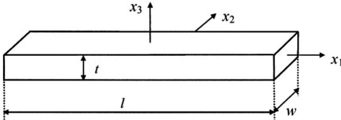
Figure 4.7-1. A piezoelectric rod with rectangular cross section.
