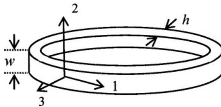
Figure 4.8-1. A ceramic ring with radial poling.
