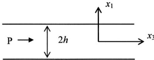
Figure 4.2-1. An unelectroded ceramic plate with in-plane poling.
