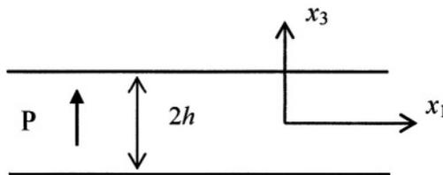
Figure 4.2-2. An unelectroded ceramic plate with thickness poling.
