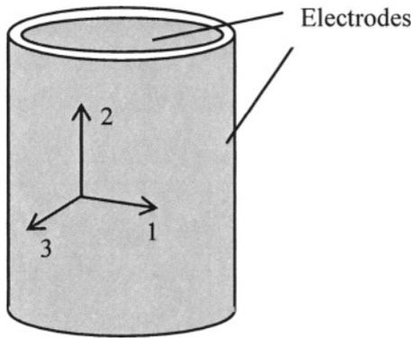
Figure 4.10-1. A thin ceramic circular cylindrical shell.
